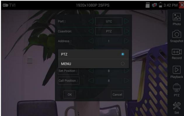
Input calling dome camera menu address code, after finishing the parameter settings, you can press the key
