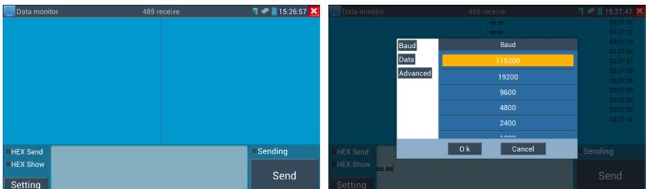
Click "Setting" to choose the baud rate of RS485/RS232; it must be the same as the DVR or the Control keyboard .The DVR or Control keyboard send the code to the tester, if it can be read, the protocol will shown on the upper right, like Pelco D, if not, like P:---
