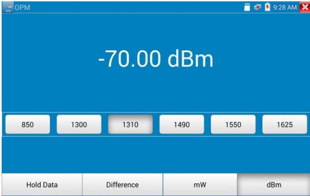
**Relative power value (optical link loss) measurement**
