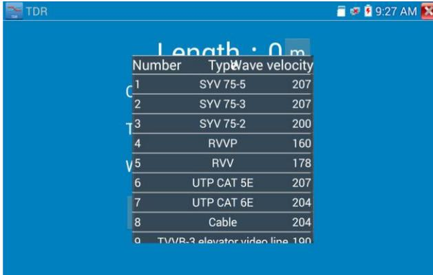
User-defined calibration: Choose the cable 100 meters to 200 meters (more than 50 meters) , click “Cable” , “Type” to select user-defined 1 for calibration, 11 groups user-defined can be set.
