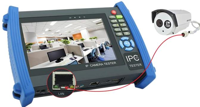
**Note:**1) If the IP camera requires PoE power, then connect the IP camera to the IP tester's LAN port . The tester will supply PoE Power for the IP camera. Click on the icon labeled POE to turn the PoE Power off or on.
