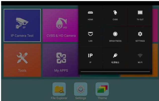
**HDMI:** Click HDMI IN to enter , In HDMIN mode, It can converter test from analog to digital with dual test window IP & HDMIN or Analog & HDMI in
