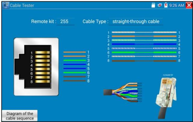
Test LAN cable or telephone cable.
