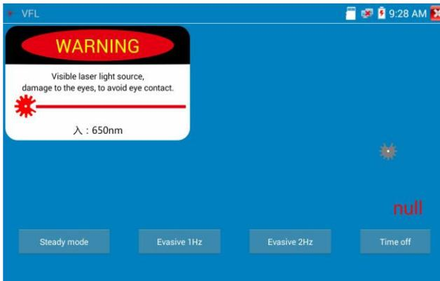
VFL four status can select——“Steady mode”, “Evasive 1Hz”, “Evasive 2Hz”and“Time off”. Click button “Steady mode” to enter steady status, click button “Evasive 1Hz” and “Evasive 2Hz, to enter pulse mode, click button “Time off”, VFL is turned off. Timed turn off can select (5 mins, 10 mins, 30 mins, 60 mins and 120 mins).
