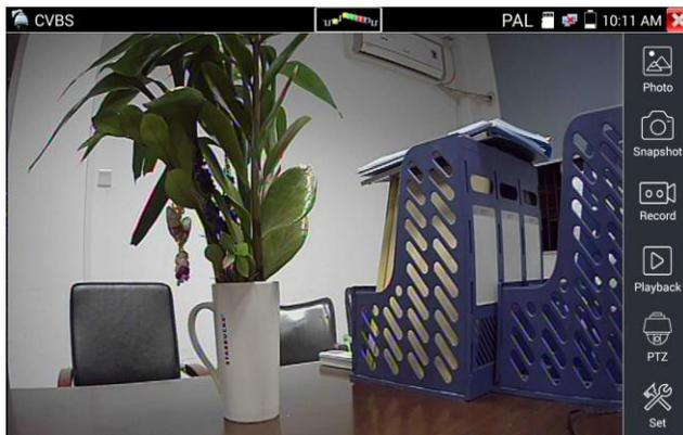
Display the input video image, click the top menu bar icon
