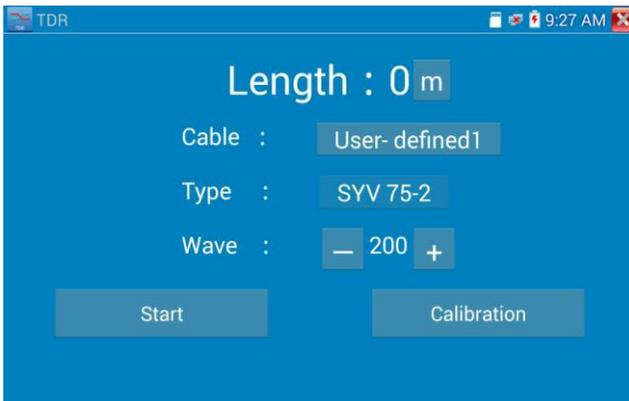
1. Select user-defined and click “Calibration” to enter test , click “user-defined 1” can define cable name, such as: AiPu BNC-5
