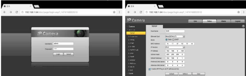
The IP camera and IP tester be on the same network segment for the browser to interface with the camera. If they are not in the same segment, click the button
