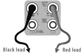
c. Connect test red lead across to the anode, the black lead to the cathode of the diode under testing.
