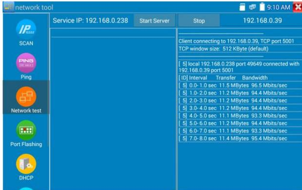
Or use tester as a Server, computer as test Client ( select Client, input tester's IP address to test)
