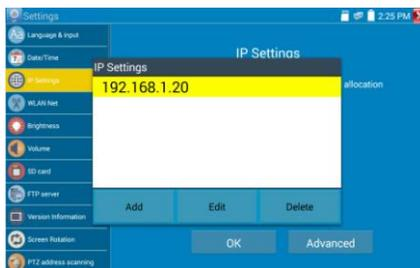
After setting an advanced IP address (refer to the photos above), the unit can test two network segments (192.168.5.0) and (192.168.1.0)
