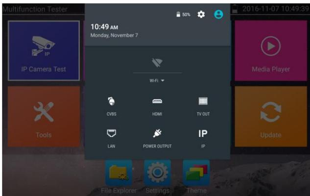
**HDMI:** Click HDMI IN to enter, In HDMI IN mode, it can convert test from analog to digital with dual test window IP & HDMI in or Analog & HDMI in.
