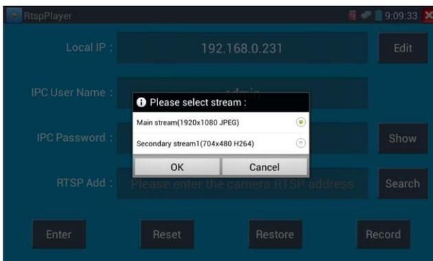
**Note:** in the event the ip tester does not auto detect the rtsp stream, refer to the specific camera manufacturer for the specific rtsp stream url. you may find this on line with a search of the camera model number and the word rtsp.
