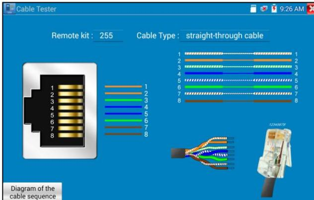
Test LAN cable or telephone cable.
