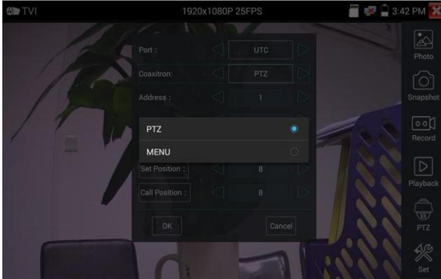
Input calling dome camera menu address code, after finishing the parameter settings, you can press the key **ENTER** or click the icon
