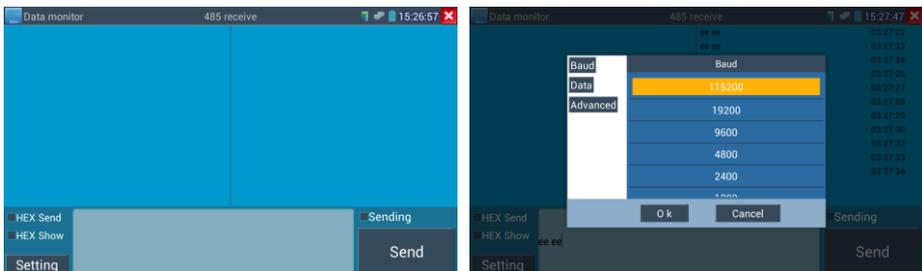
Click "Setting" to choose the baud rate of RS485; it must be the same as the DVR or the Control keyboard .The DVR or Control keyboard send the code to the tester, if it can be read, the protocol will shown on the upper right, like Pelco D, if not, like P:--
