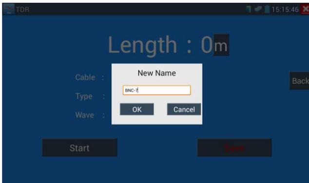
**Application:** TDR test is the use of pulse reflection method, to transmit pulse signal for tested cable, when cable is open circuit or short-circuit, reflected pulse is generated, the tester receives and deals with the reflected wave, measurement results displayed on the screen. TDR can test cable open circuit and short circuit, help engineer quickly find the cable’s problem location. It is more convenient and efficient to repair the faulty cable.
