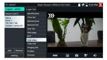
**IP camera video settings:** Click "Video Set" to enter the IP camera's encoder and resolution settings. Make the desired changes and click "OK" to save.
