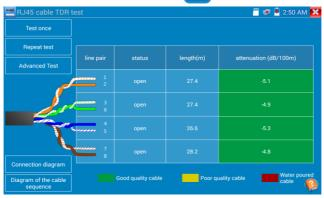
**Single test:** Test cable status, length and attenuation.
