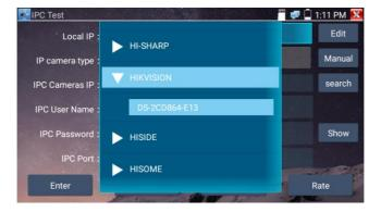
**Stream code:** When test camera via RTSP, you can select mainstream or sub stream to test (if camera's RTSP have not been start or without, it will tip "auto match" fail, please witch to manually selecting
