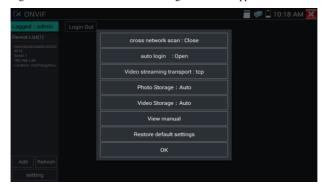
Across network segments scan: After open this function, enter "Setting"-"IP Settings"-"Advanced" to add other network segments IP, Rapid ONVIF function can across network segments to scan camera's IP.
