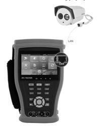
Note:1) If the IP camera requires PoE power, then connect the IP camera to the IP tester's LAN port.
