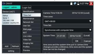
Maintenance: For camera software reset or restore to factory settings.
