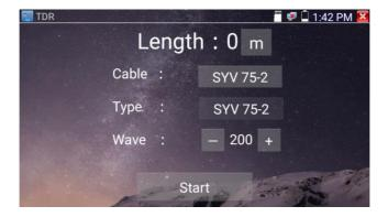
Built-in BNC cable, network cable, RVV control cable, Telephone line and TVVB cable etc can test. 11 groups user-defined cable can be set.
