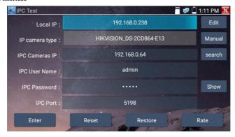
**Local IP**: This is the tester's IP address. Click "Edit" to enter "IP setting" and change the tester's IP address settings
