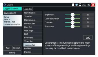
**Profiles:** Click "profiles", can view video streaming current configuration files, as well as switch between Major stream and minor stream.
