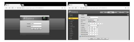
The IP camera and IP tester be on the same network segment for the browser to interface with the camera. If they are not in the same segment, click the button or press "RETRUN" to exit. Open the "Settings" app from the main menu to change the IP tester's network settings to match those of the IP camera
