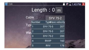
User-defined calibration: Choose the cable 100 meters to 200 meters (more than 50 meters), click "Cable", "Type" to select user-defined 1 for calibration, 11 groups user-defined can be set.
