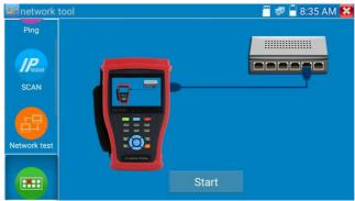
If the tester and PoE switch are connected well, the LAN port of POE switch flash at special frequency, If not, no any changes on the LAN port
