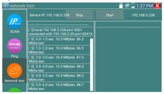
b). Start send packet test: Using the other IP tester, type in the Server's IP address at the top right corner of the screen. This app is used to send packets for network speed testing. Click the "Start" button to send the packets and start testing.
