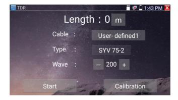
1.Select user-defined and click "Calibration" to enter test , click "user-defined 1"can define cable name, such as: AiPu BNC-5
