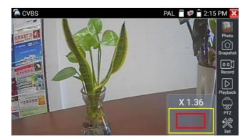
If not use touch screen to operate, press the key TELE+ to zoom out , press the key WIDE- to zoom in, press upward and downward key to move the image
