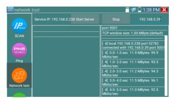
Or use tester as a Server, computer as test Client (select Client, input tester's IP address to test)
