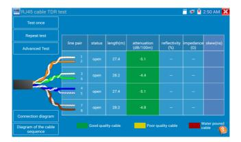
**Advanced Test:** Test cable pair status, length, attenuation, reflectivity, impedance, skew and other parameter.
