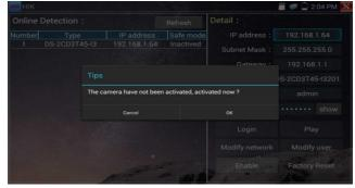
2.Input password: Input new password, tap "ok" to activate
