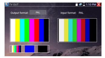
**BNC loop test:** Tester can send and receive color bar generator through the tester's "video out and video in" port, it is for testing transmission channels, such as video Optical, video cables etc. The tester "VIDEO OUT" port to connect optical terminal's sending port, and "VIDEO IN" Port to optical
