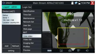
When the image is enlarged, if not operate on touch screen, it can operate by the keyboard , press the key TELE+ to zoon in , press the key WIDE- to zoom out , press upward and downward key to move image.
