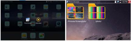
The Media player can browse video and image files. It supports the video formats of MP4, H.264, MPEG4, and MKV. The IP tester recorded files can play directly via the Media player. The Media player will automatically display the video files from the SD card. Click on the desired file to play. Click RETURN to exit.
