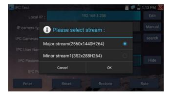
**IP Camera's IP:** Enter the IP camera's IP address manually or click "Search" to auto-scan for the IP camera's IP address. It is better to directly connect the IP camera to the tester so the search results will only display the camera's IP address. If the tester is connected to a PoE switch, it will find and display several IP address
