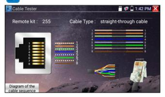
Test LAN cable or telephone cable.
