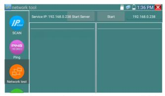
a).Start the server: Click "Start Server" button to use the tester as a Server. It will display its IP address at the top of the screen.
