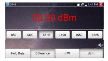
Data hold and Relative measuring use together, the data is yellow while the function is effect.
