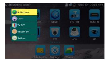
Press the key "MENU", you can turn on it and switch functions, then press ( to enter app, tap other area on the screen, to exit the menu
