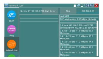
Network bandwidth testing can also be tested with a computer using compatible network bandwidth testing software. Install network bandwidth testing software on a computer, as a test Client or Server, to do the mutual testing with the tester. If use computer as the server, the computer IP address is:192.168.0.39
