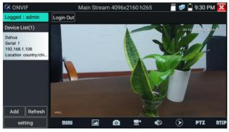
If you select ONVIF Rapid mode, the meter automatically scan different network segments for ONVIF cameras. It lists the camera name and IP address on the Device List. Tester can auto login camera and display camera image.
