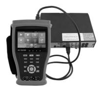
DVR or other device's HDMI out port connect to tester's HDMI in port, the meter will display input image
