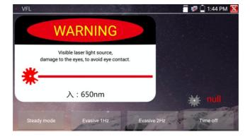
VFL four status can select——"Steady mode", "Evasive 1Hz", "Evasive 2Hz" and "Time off". Click button "Steady mode" to enter steady status, click button "Evasive 1Hz" and "Evasive 2Hz", to enter pulse mode, click button "Time off", VFL is turned off. Timed turn off can select (5 mins, 10 mins, 30 mins, 60 mins and 120 mins).
